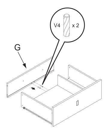
2. Attach back board (G) to the drawer with wooden dowels (V4).
